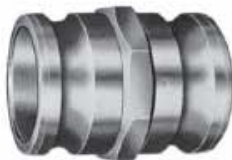
Part SA spool adapter connects two lengths of hose with coupler ends. 1/2" to 6". In all metals except in large sizes. (Spool couplers are also available.)
